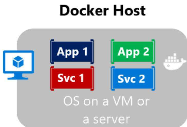
Figure 2-1. Multiple containers running on a container host
