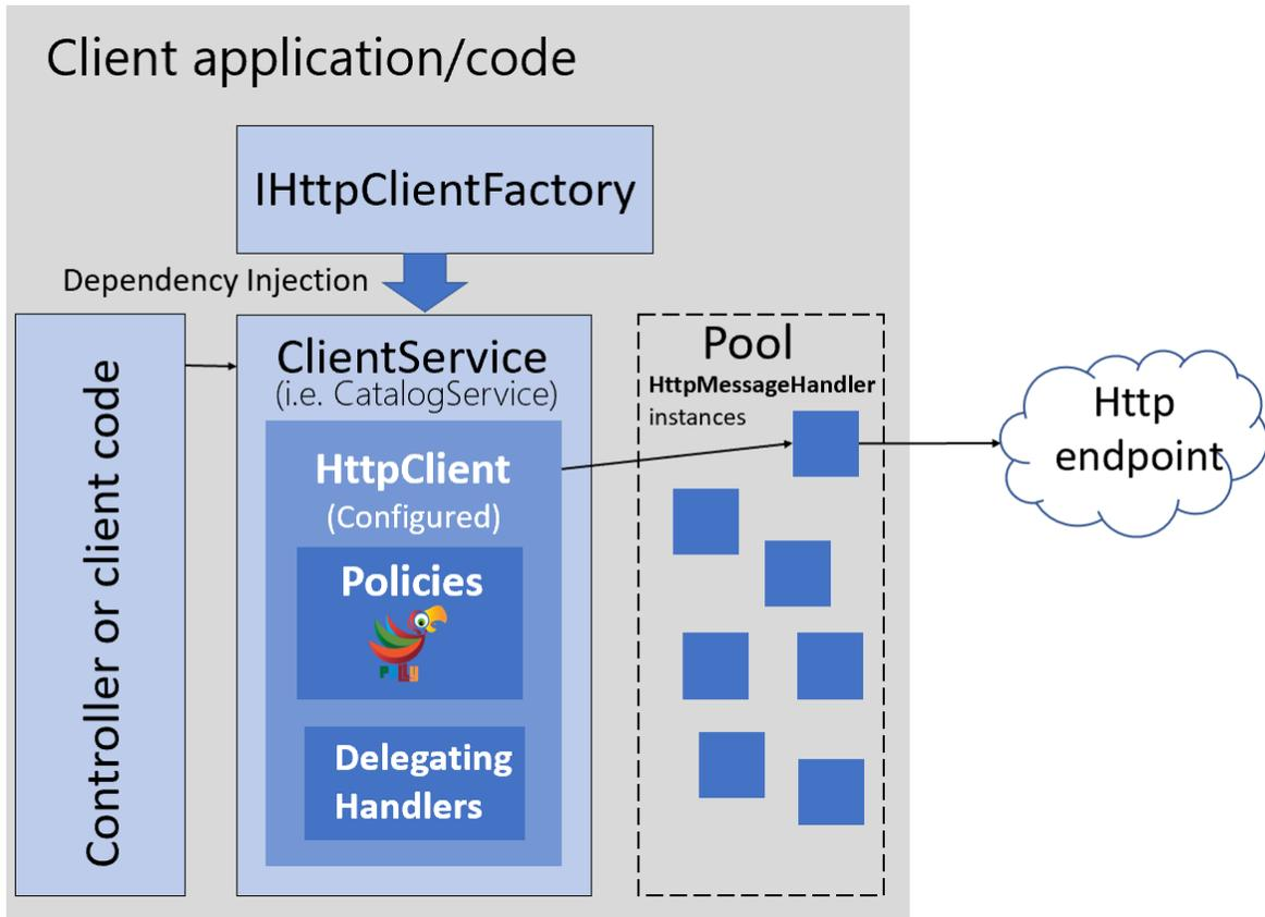
Figure 8-4. Using IHttpClientFactory with Typed Client classes.
