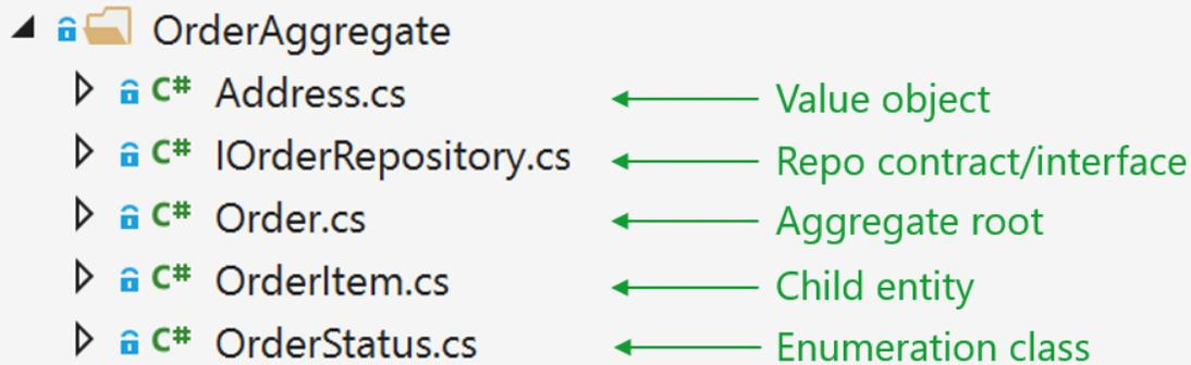
Figure 7-11. The order aggregate in Visual Studio solution
