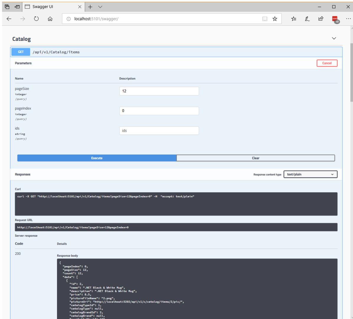
Figure 6-9. Swashbuckle UI testing the *Catalog/Items* API method
