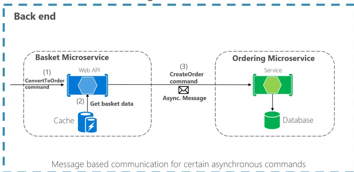
Figure 4-18. A single microservice receiving an asynchronous message
