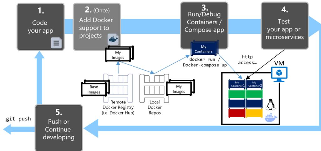
Figure 5-15. Simplified workflow when developing with Visual Studio
