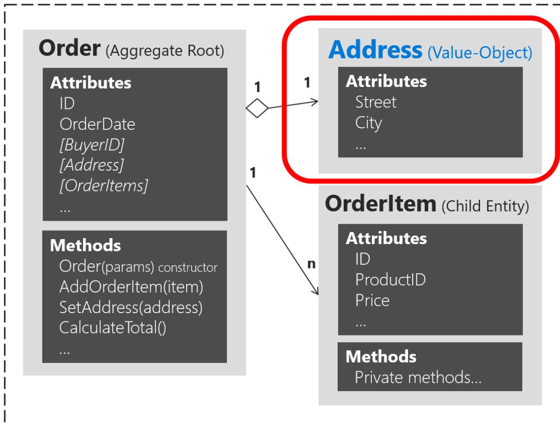
Figure 7-13. Address value object within the Order aggregate
