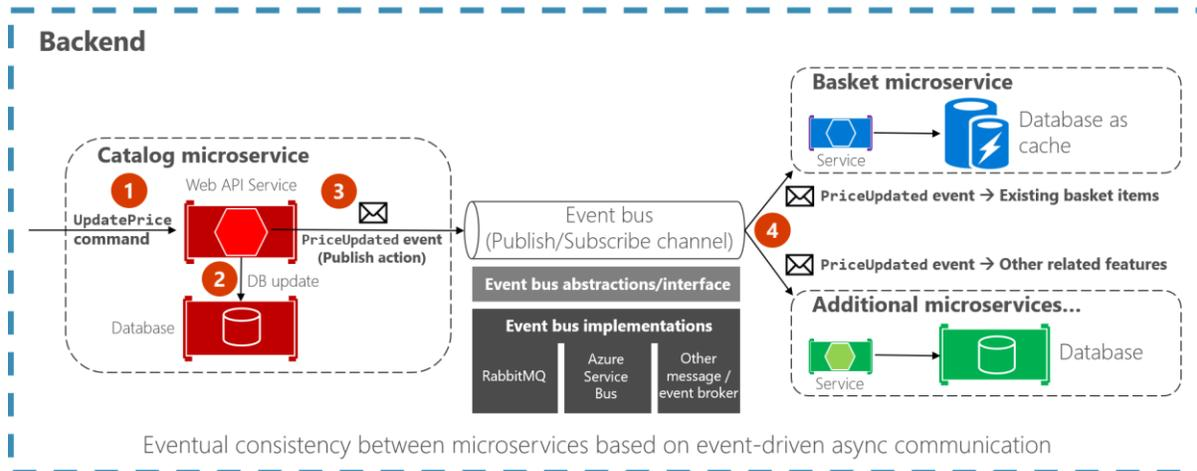
Figure 6-18. Event-driven communication based on an event bus
