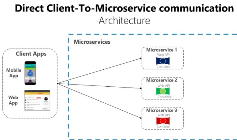
Figure 4-12. Using a direct client-to-microservice communication architecture
