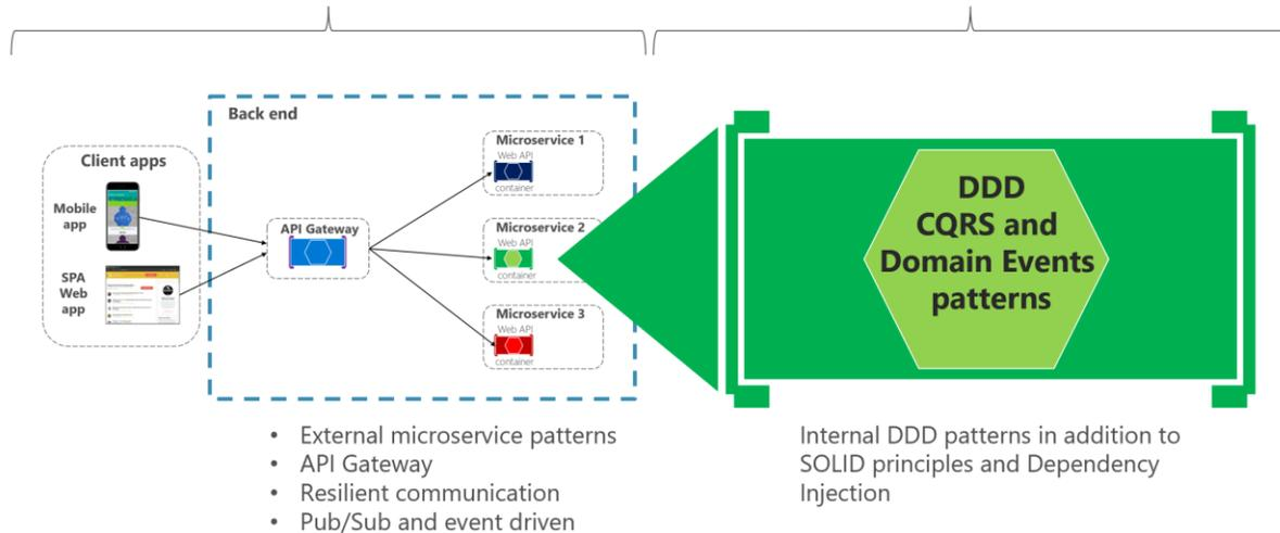
Figure 7-1. External microservice architecture versus internal architecture patterns for each microservice
