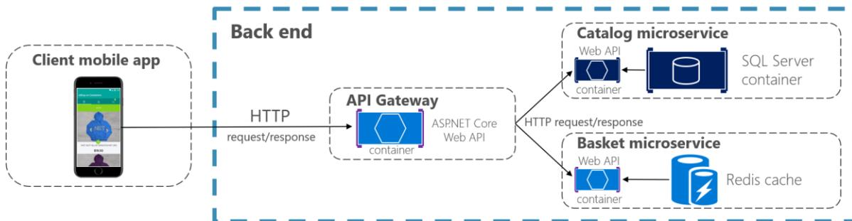
Figure 4-16. Using HTTP request/response communication (synchronous or asynchronous)
