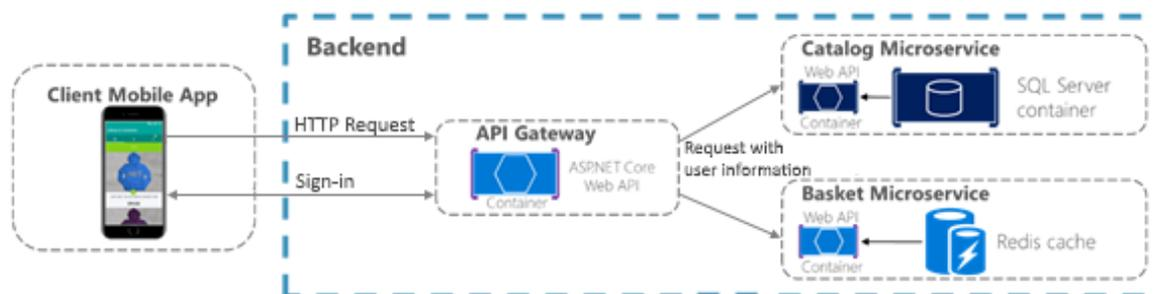
Figure 9-1. Centralized authentication with an API Gateway
