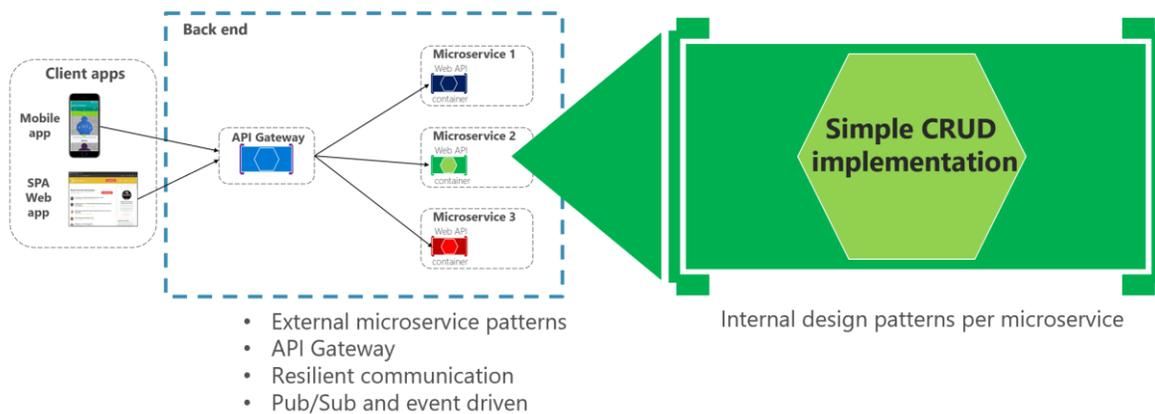
Figure 6-4. Internal design for simple CRUD microservices
