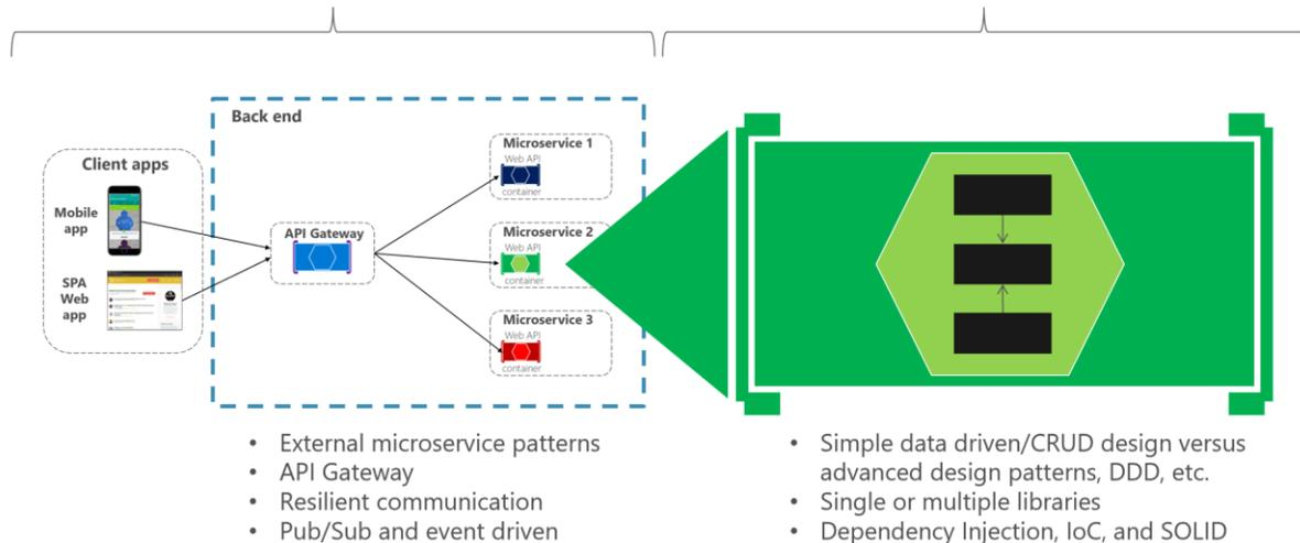
Figure 6-2. External versus internal architecture and design
