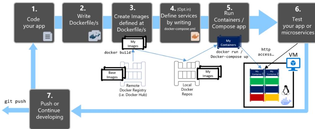
Figure 5-1. Step-by-step workflow for developing Docker containerized apps
