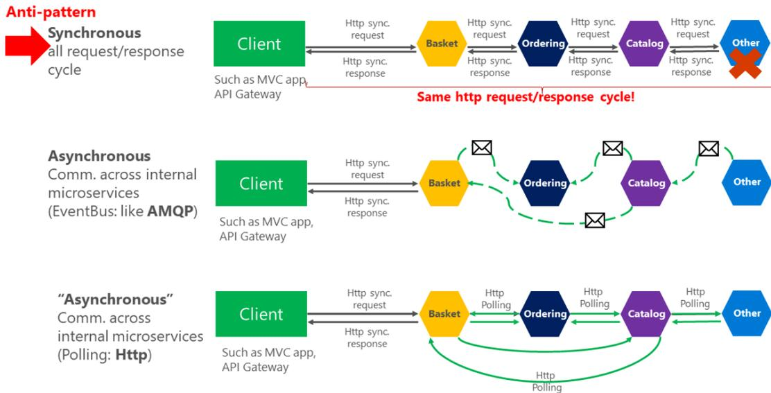
Figure 4-15. Anti-patterns and patterns in communication between microservices
